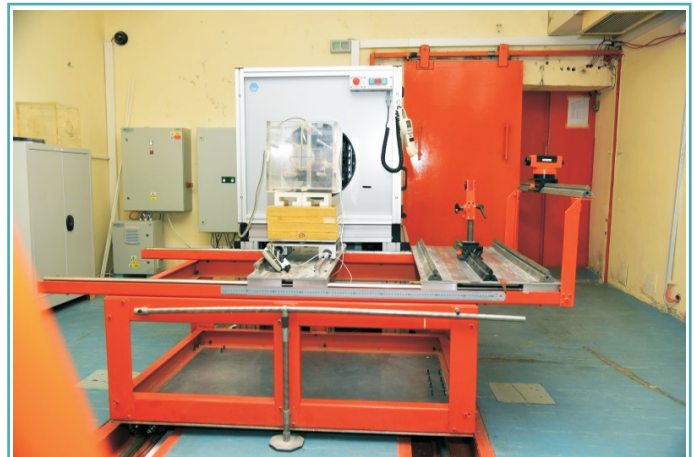
Absorbed dose rate calibration set-up in front of newly installed Co-60 therapy level calibrator
