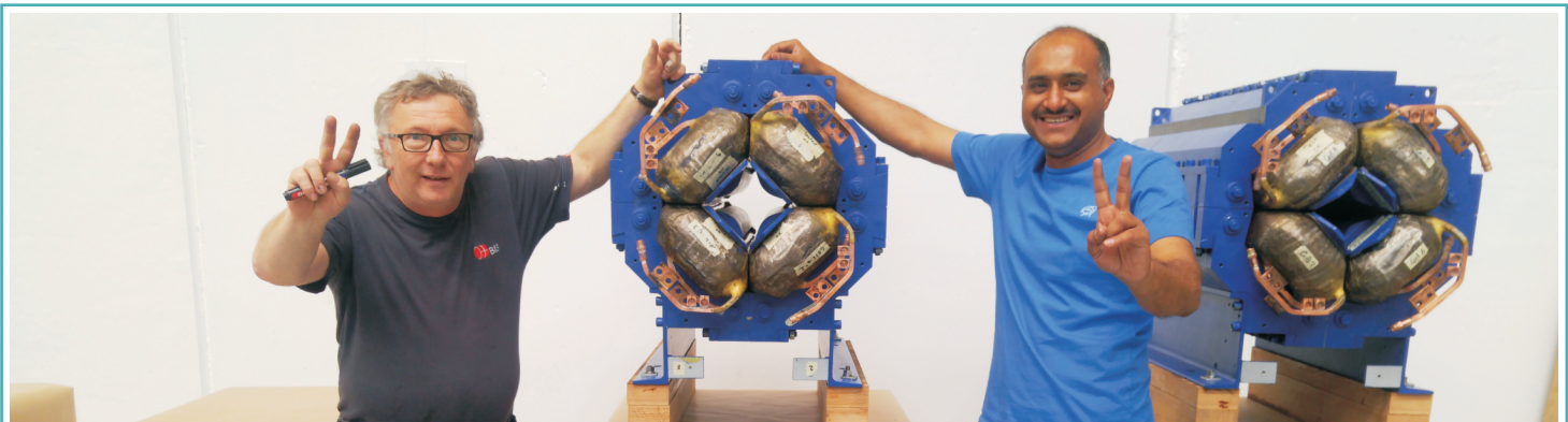
First two magnets disassembled and then assembled successfully after renovation at CERN
